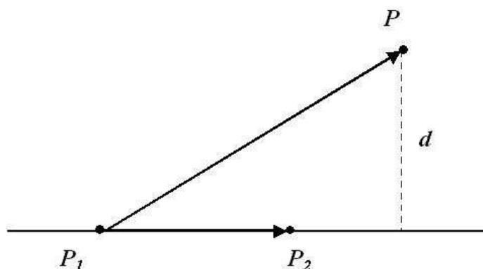
$$\begin{aligned} \vec{P_1P} &= 5\vec{u}_x - 3\vec{u}_y + 5\vec{u}_z \\ \vec{P_1P_2} &= 2\vec{u}_x - 1\vec{u}_y + 4\vec{u}_z \end{aligned}$$
