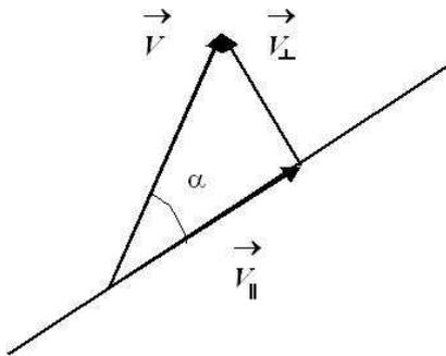
$$V_{\parallel} = |\vec{V}| \cos \alpha \quad V_{\perp} = |\vec{V}| \sin \alpha$$
